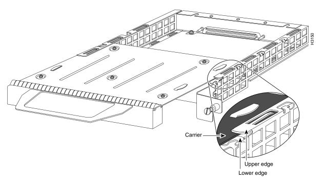
Step 11 Carefully slide the new port adapter into the port adapter slot until the connector on the port adapter is completely mated with the connector on the motherboard.
